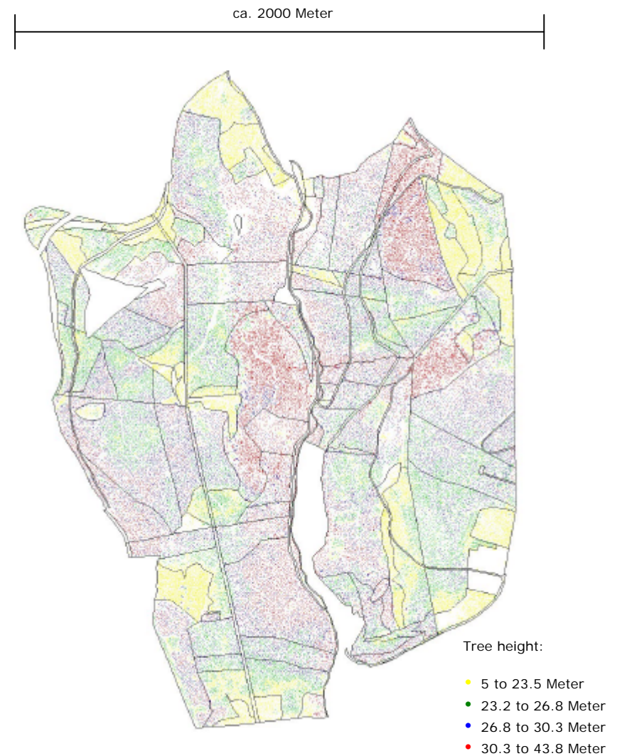
Fig. E2: Some 95.000 trees have been automatically detected, classified and height measured. The algorithm used is robust and suitable for processing several thousand hectares.
