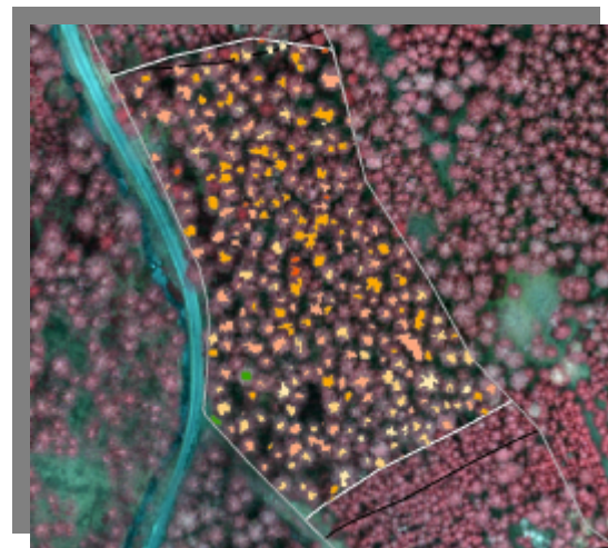
Fig. B1: Crown Centroids with different colours for different chlorophyll activity (NDVI Value)
