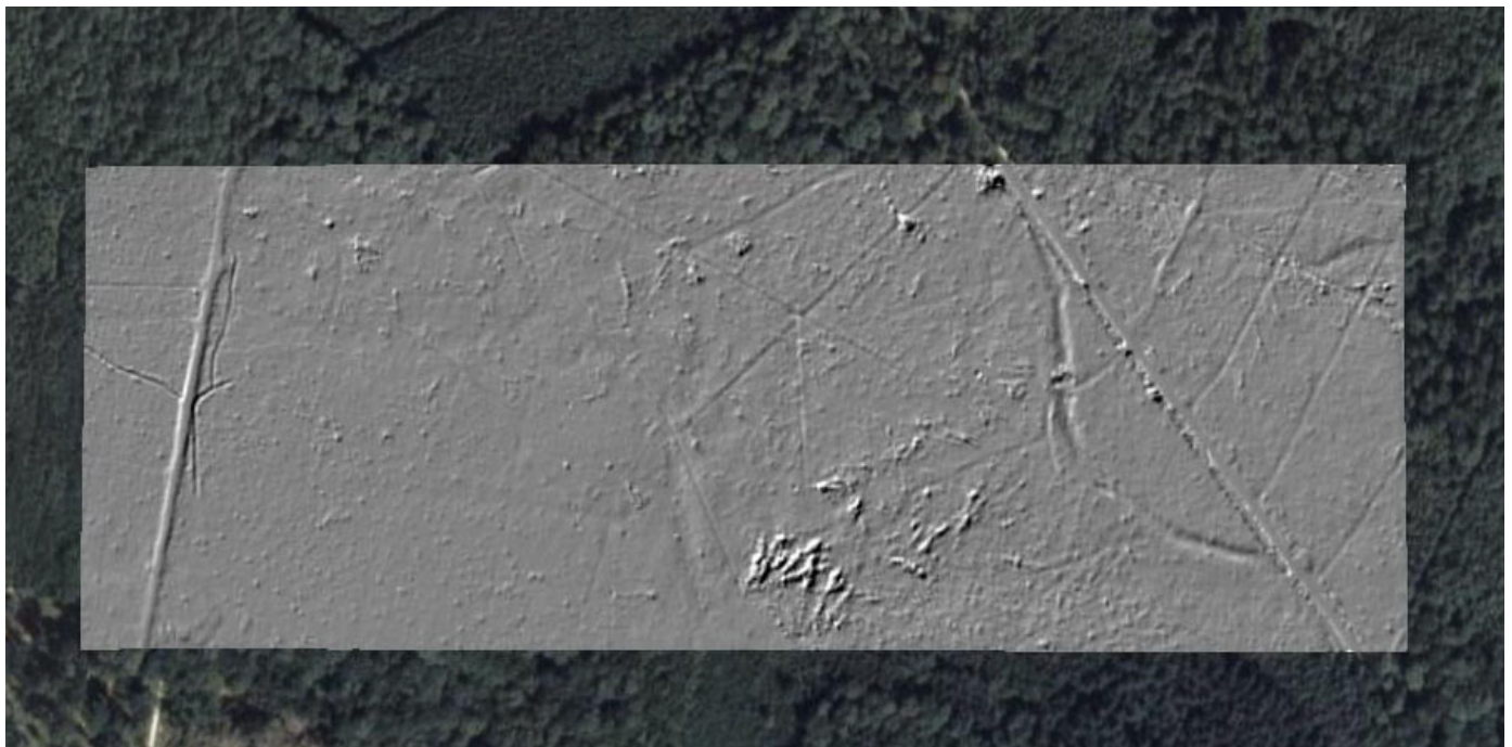
Fig. 7: The terrain model (grey rectangle) generated from the raw LiDAR point data shows hidden structures under the forest cover (green background area). © TopoSys, landConsult.de.
