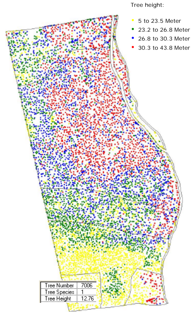
Fig. D4: Individual tree tops and tree height after processing the nDSM with a local maxima algorithm. From the individual tree heights, the mean average height of all trees and the maximum height of the hundred highest trees per ha and per stand will be calculated.
