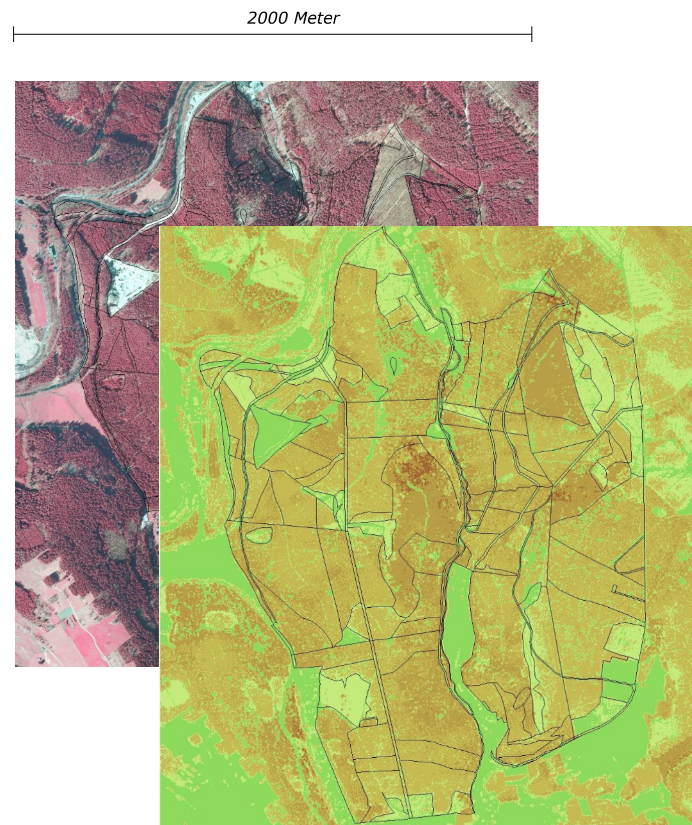
Fig. E1: Standard CIR Ortho Mosaic and LiDAR Data have been processed to assess the wood volume on some 250 ha mixed forests.
